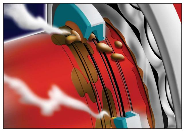
Rubber lip seals effectively perform for, on average, 1844 hours and consume 147 watts of power while they're sealing, according to industry sources. They groove the shaft and heat the bearing lube.
